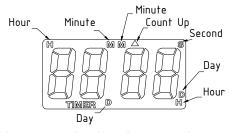
" $\Delta$ " – flashing means the timer is at counting mode; steady displayed means it is at stop mode.
