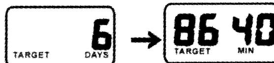
F. In order to allow you precise managing of your Target, when the counting reaches to 150 minutes, the clock automatically change the display format from minutes to seconds.
