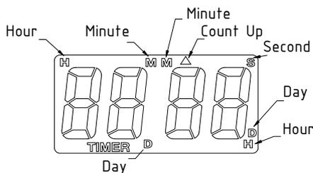
“Δ” – flashing means the timer is at counting mode; steady displayed means it is at stop mode.
