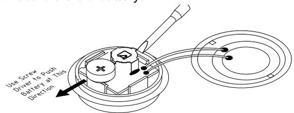
4. Insert a fresh battery (positive side up) into the metal holder.
